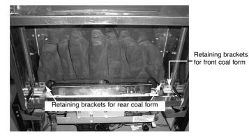
b) Fit the front ceramic coal form in front of the burner, as shown below in Fig 6. Ensure that the front ceramic coal form is correctly located behind the retaining brackets at the L/H & R/H ends.
